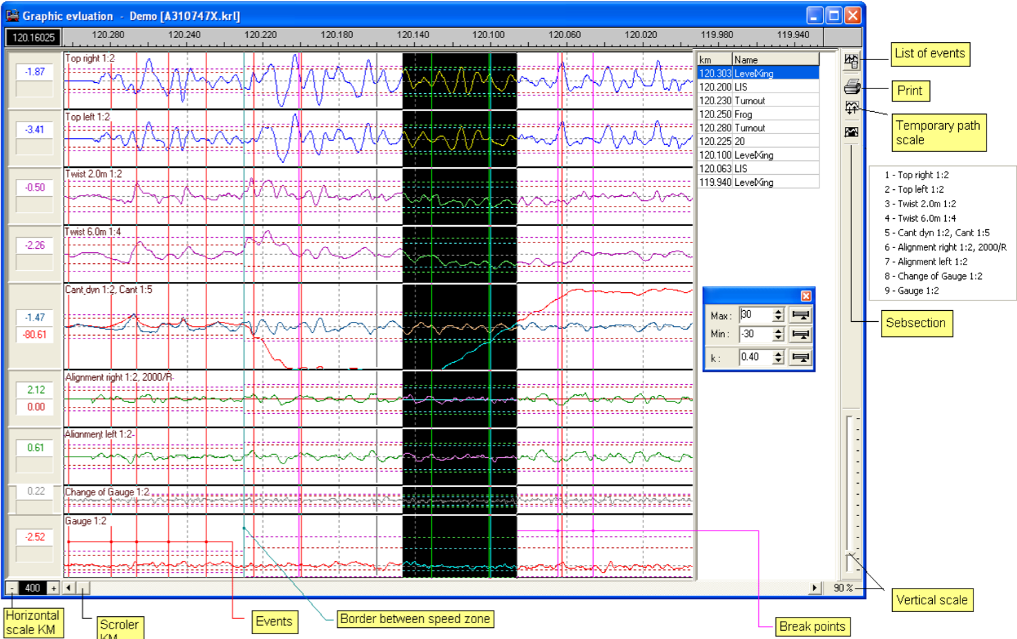
The example of track geometry graph printed by assessment software
