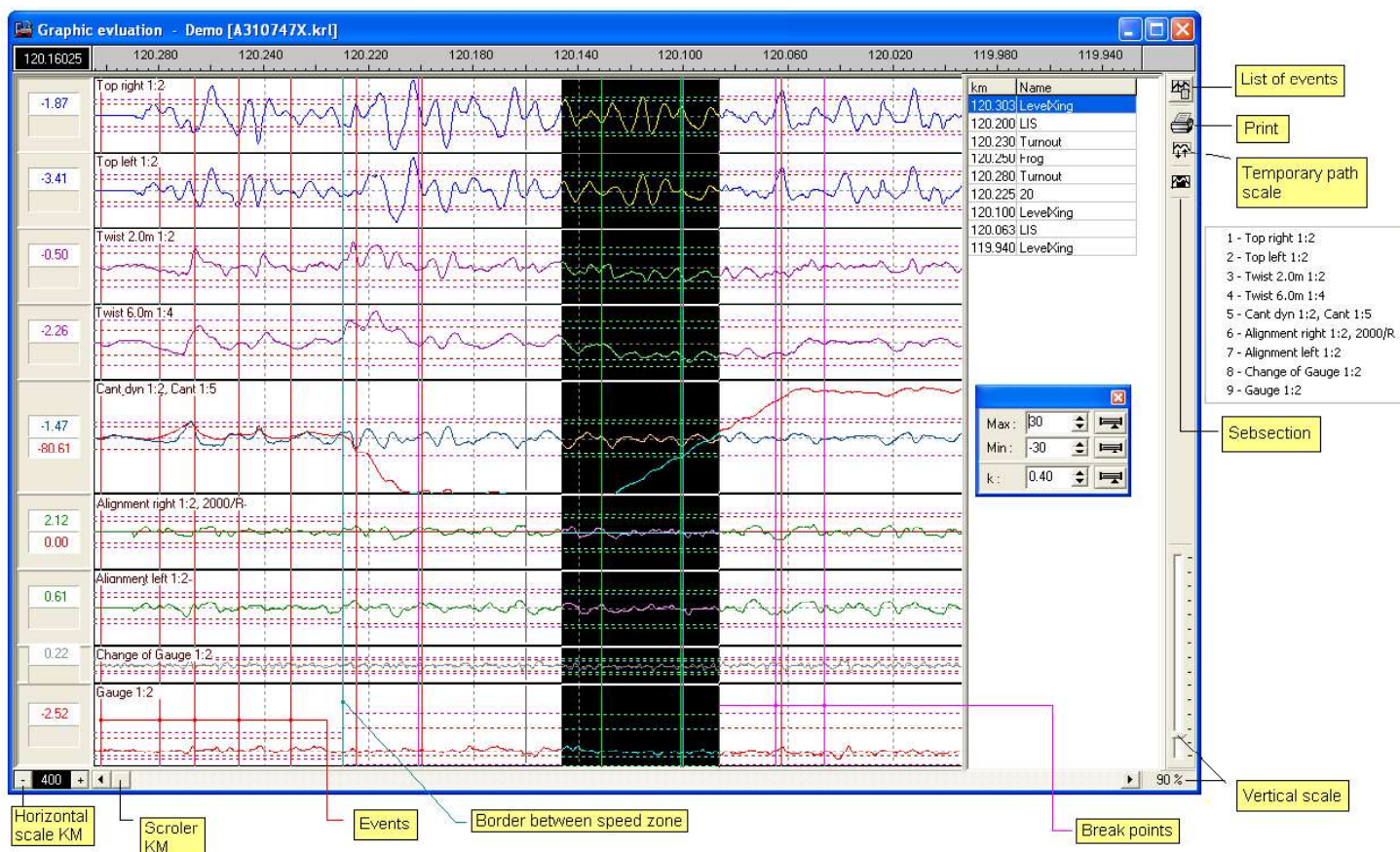
The example of track geometry graph printed by assessment software
